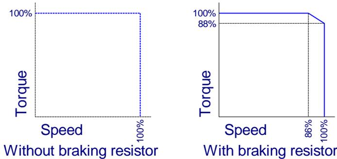
One side benefit of providing a braking resistor is the extended brush life of the motors. The braking resistor tends to suppress the arcing of the brushes and commutators.
