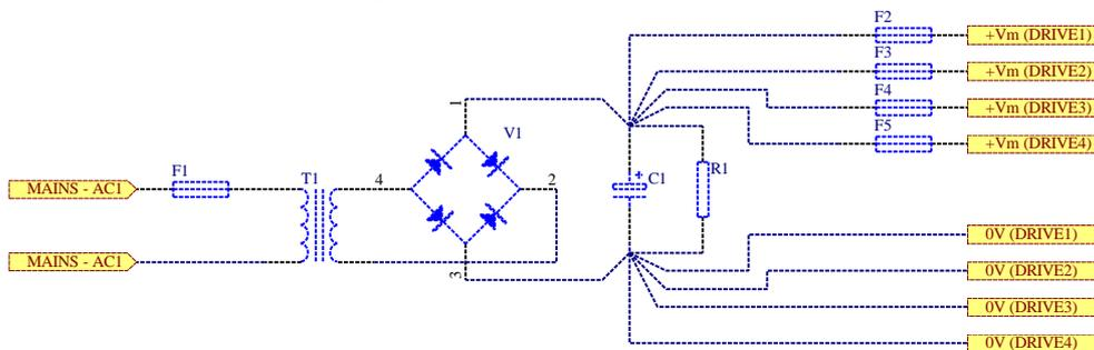
To minimize ground loops, the Vm voltage should be distributed in star configuration directly from the terminals of the capacitor and individually fused.
